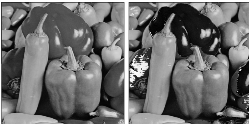
Fig. 1. Luma components of the “peppers” image after RCT (left) and mRCT (right) transformations.
